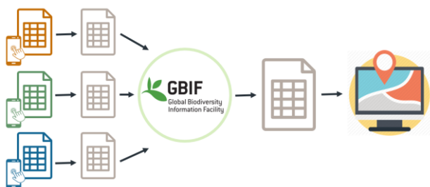
Figure 19: Illustration of the data flow from data collection via smartphone application and publication on GBIF to visualization on the dashboard.
