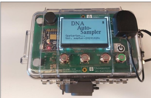
Figure 8: eDNA autosampler for automated water sampling.
