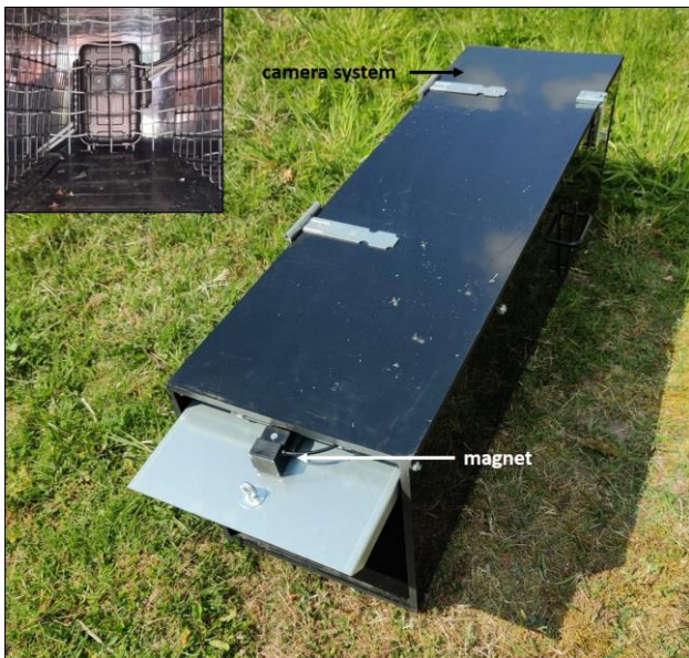
Figure 14: Composition of the prototype of the selective life traps with electromagnet at the door and image recognition system in the rear part of the trap. Inserted picture: image recognition system in the trap.
