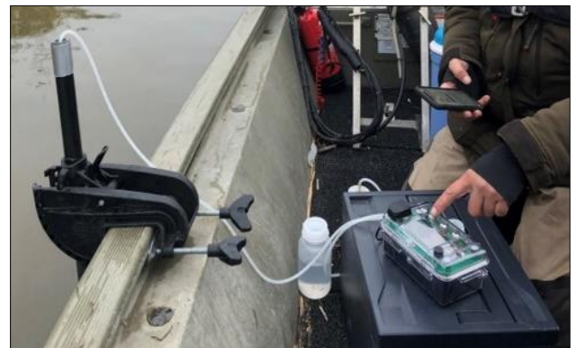
Figure 9: Water sampling via eDNA autosampler from a boat. The water samples run through a plastic tube and are collected in a plastic bottle.
