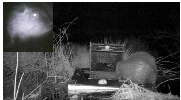
Figure 16: A coypu enters the smart life trap. The inserted picture shows an image taken of the animal by the camera inside of the trap. The image is directly analyzed and classified by the algorithm.
