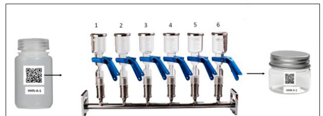
Figure 10: Processing of the water samples. The water from the plastic bottle is filtered and the filter paper containing the eDNA is further processed.
